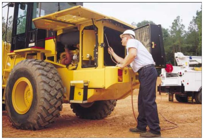
Easy, Wide Open Access. Gull-wing engine enclosure doors with pneumatically-assisted lift cylinders effortlessly lift up for exceptional access to major power train components. All filters and service points are within easy reach.
